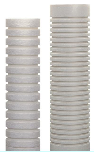
RB (Resin-Bonded) Cartridge is produced from cellulose fibers, which have been intrinsically bonded together by a melamine resin, to create a solid highly durable & porous structure. By treating the fibers in this fashion we can ensure a stronger cartridge that is less likely to collapse than a wound or pleated cartridge.
